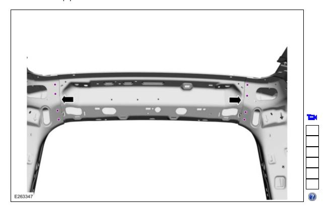
4. Break the adhesive bond and remove the roof rear frame.
