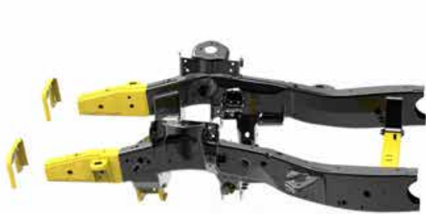
Front-Third Frame Section Top view
